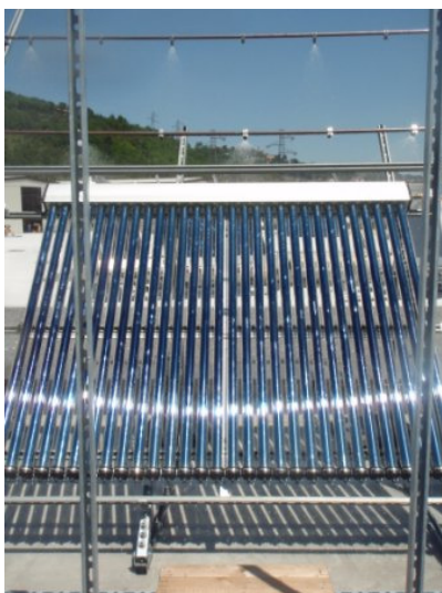
Fig. 3: rain penetration test
