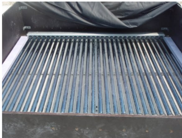
Fig. 2: mechanical load test
