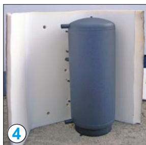
4 Only mount insulation when pre-heated! Pre-heat it for 24 hours to at least of 22 °C.
